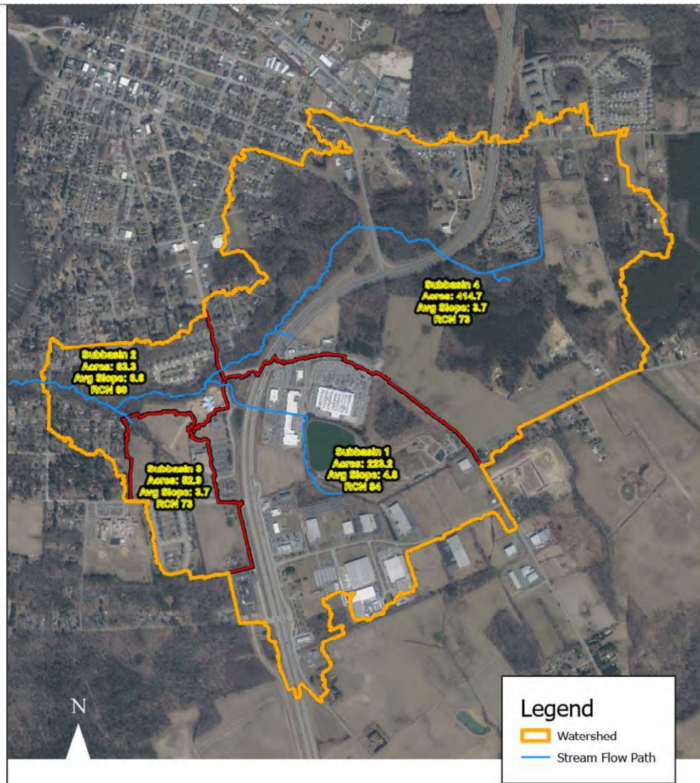
Figure 11. Sub-basins within the Poor House Run watershed that were used for the hydrologic analysis
