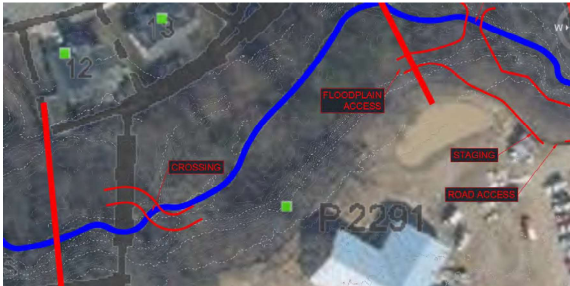
Figure 3. Phase 2 Access / Staging Map
